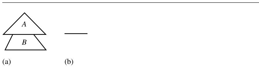
Figure 13.28 (a) Two polygons that are reported not to intersect by the pseudocode. (b) The actual set intersection, a line segment.
